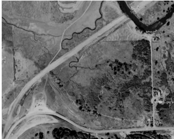
Figure 81. Fraser Creek was cut in two by U.S. Highway 101. A ditch was dug parallel to the highway on the southeast side to connect the upstream portion of Fraser Creek to the Salmon River. The downstream section of Fraser Creek is just northwest of U.S. Highway 101 and was left as a remnant channel.
