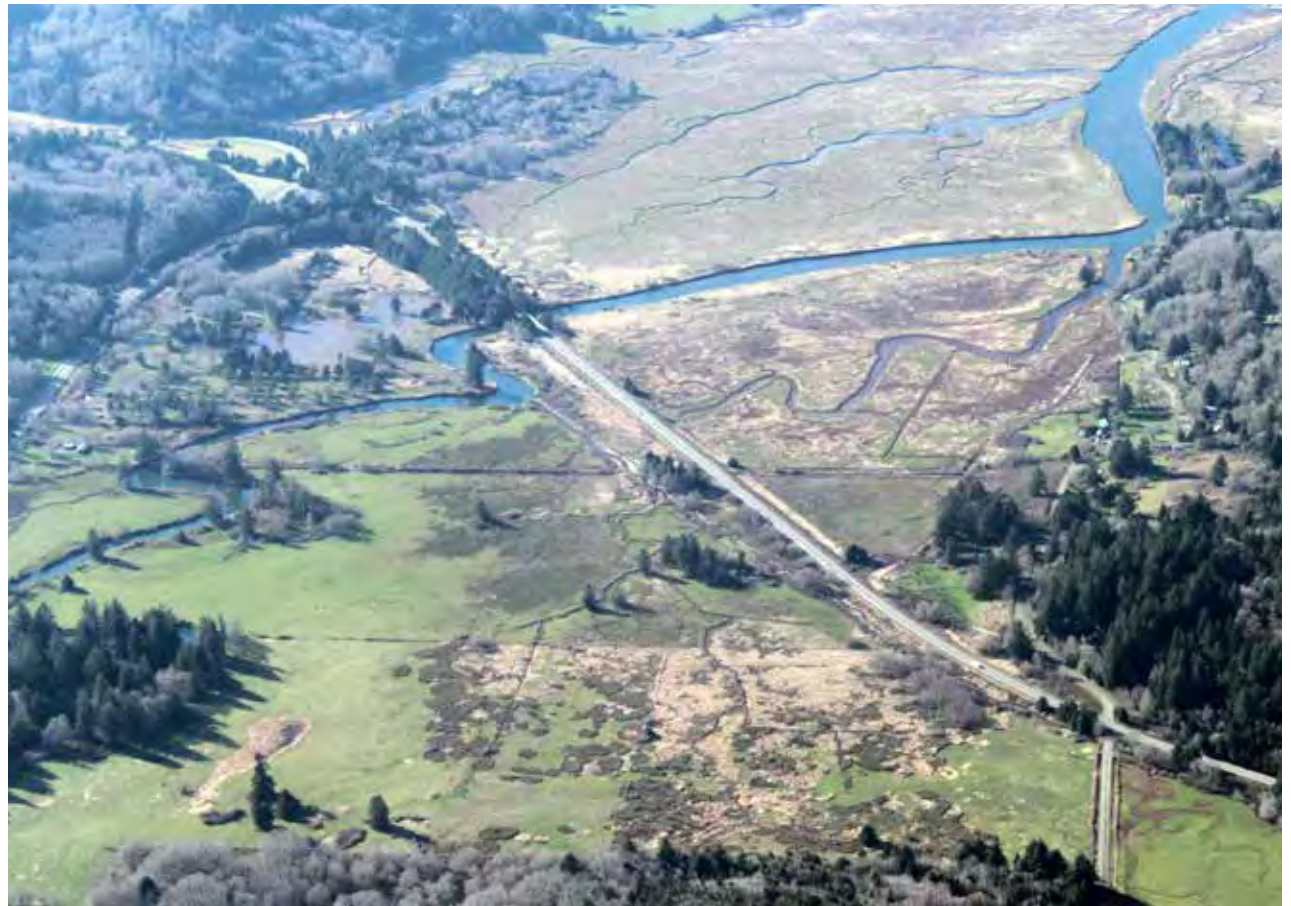
Figure 80. 2011 aerial photo of U.S. Highway 101. Since 1961 Salmon Creek has been rerouted into the ditch (parallel to U.S. Highway 101). The historic Salmon Creek (to the right of U.S. Highway 101 and below Salmon River) is truncated by the highway. Photo credit Anthony Veltri.
